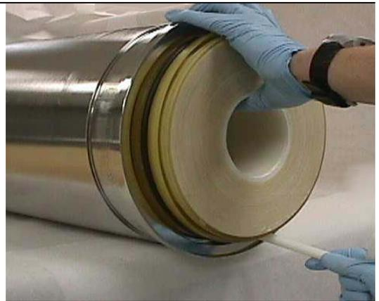
**After the O-ring has been inserted where these arrows point, use the insertion tool as pictured. Carefully tap with rubber mallet to complete O-ring insertion.**
