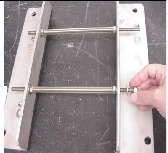
The equipment illustrated above is required for the assembly or disassembly of a 10X28 Liqui-Cel Membrane Contactor with sanitary connections that will be assembled in a 316L SS Housing.
